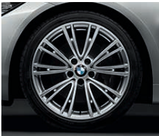
□ 19" BMW Individual light alloy wheels V-spoke style 626 I with mixed tyres, 8 J x 19, 225/40 R 19 tyres at the front, 8.5 J x 19, 255/35 R 19 tyres at the rear. Discreet, laser-engraved BMW Individual logo. 2
