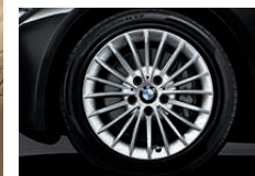
■ 17" light alloy wheels Multi-spoke style 414 with 7.5 J x 17, 225/50 R 17 runflat tyres.
