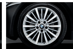
□ 18" light alloy wheels Multi-spoke style 416, highly polished, with 8 J x 18, 225/45 R 18 runflat tyres (standard on 328i, 328i xDrive, 335i, 335i xDrive, 325d, 330d, 330d xDrive and 335d xDrive).
