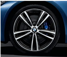
□ 19" M light alloy wheels Double-spoke style 442 M in bi-colour Orbit Grey metallic with mixed tyres, 8 J x 19, 225/40 R 19 tyres at the front, 8.5 J x 19, 255/35 R 19 tyres at the rear. 3
