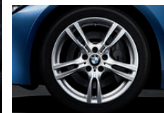
■ 18" M light alloy wheels Double-spoke style 400 M with mixed runflat tyres, 8 J x 18, 225/45 R 18 tyres at the front, 8.5 J x 18, 255/40 R 18 tyres at the rear.
