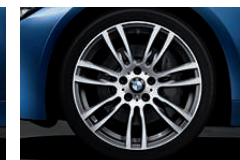
□ 19" M light alloy wheels Double-spoke style 403 M in bi-colour Ferric Grey, highly polished, with mixed runflat tyres, 8 J x 19, 225/40 R 19 tyres at the front, 8.5 J x 19, 255/35 R 19 tyres at the rear.
