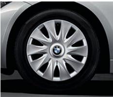
■ 16" steel wheels with full wheel covers, 7 J x 16, 205/60 R 16 tyres (standard for 316i, 316d, 318d and 318d xDrive). □ Runflat tyres (standard for 17" light alloy wheels and above).
