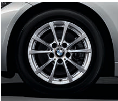
□ 16" light alloy wheels V-spoke style 390, 7 J x 16, 205/60 R 16 tyres (standard for 320i, 320i xDrive, 320d and 320d xDrive).
