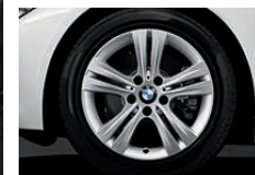
■ 17" light alloy wheels Double-spoke style 392 with 7.5 J x 17, 225/50 R 17 runflat tyres.
